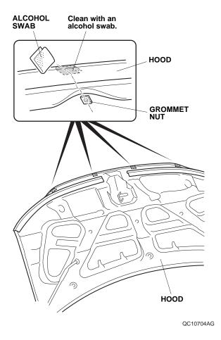
Remove the adhesive backings from the protection films, and attach them to the front of the hood area where the two brackets A and the two brackets B will mount.
