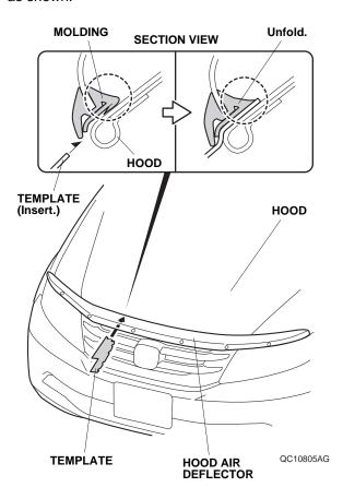
11. Open the hood. Tighten four truss screws loosely installed in step 4.
